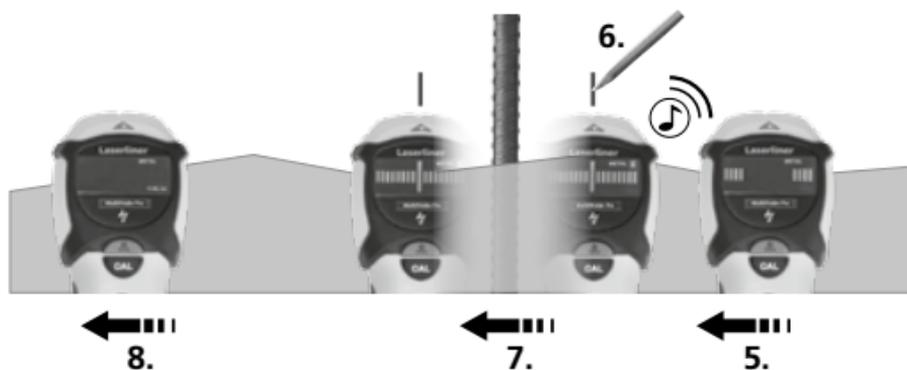
**B** **AUTO CAL PLUS** Isolate an object to be measured by passing over it several times.
