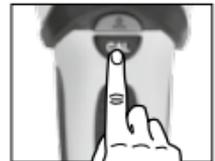
Maximum sensitivity is achieved when the device is held in the air while calibrating. This can be useful for METAL and AC-SCAN measurements.
