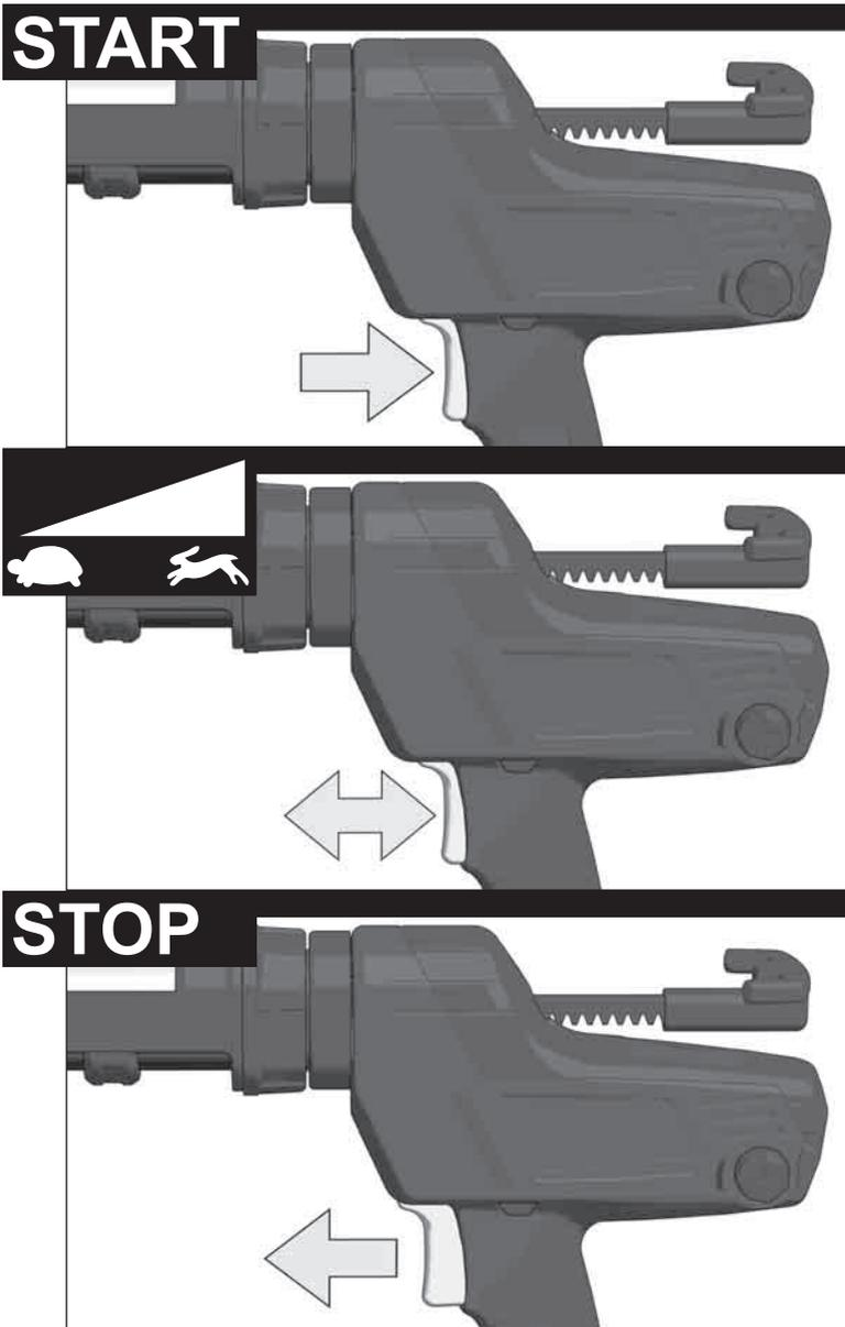
When the trigger is released, the motor will run for a short time to release the rod. This prevents a drip.
