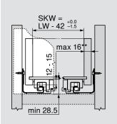
\*\* Limited side adjustment for a drawer side panel thickness of 16 mm, but with full tolerance utilisation of the SKW
