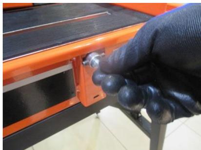
Insert 2 threaded and pinned shafts
