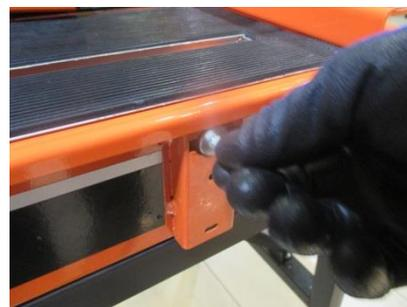
Rotate both shafts by 90°
