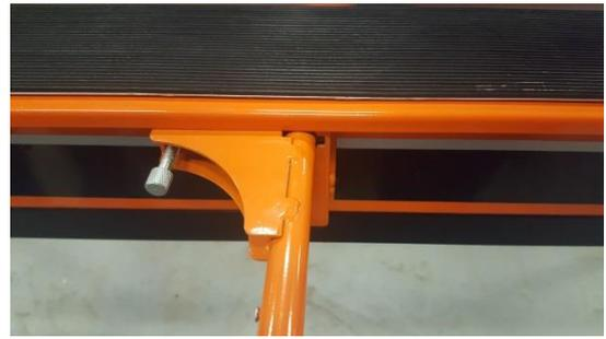
Insert both pinned shafts
