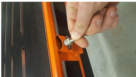
Insert 2 threaded and pinned shafts
