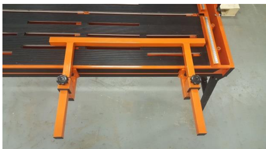
Insert the guide in both supports
