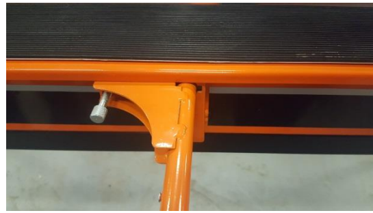
Insert both pinned shafts
