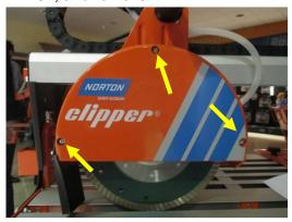
• Loosen the hexagonal nut (left threaded) on the blade shaft using the 18 mm wrench supplied with TR 202, which holds the removable outer flange.
