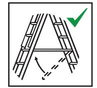
Use the ladder with restraint devices engaged
