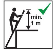
When used to access another level, ladder must extend min. 1 m over the landing point.
