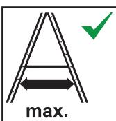
Ladder must be opened completely before use (bracing/bands should be fully opened, tightened/locked)
