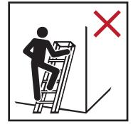
Standing ladders shall not be used as a leaning ladder unless it is designed to do so
