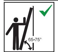
The correct erection angle for the ladder is 65-75°
