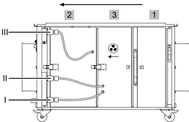
Then connect the two sensor hoses on the sensor hose side in accordance with the selected configuration:
