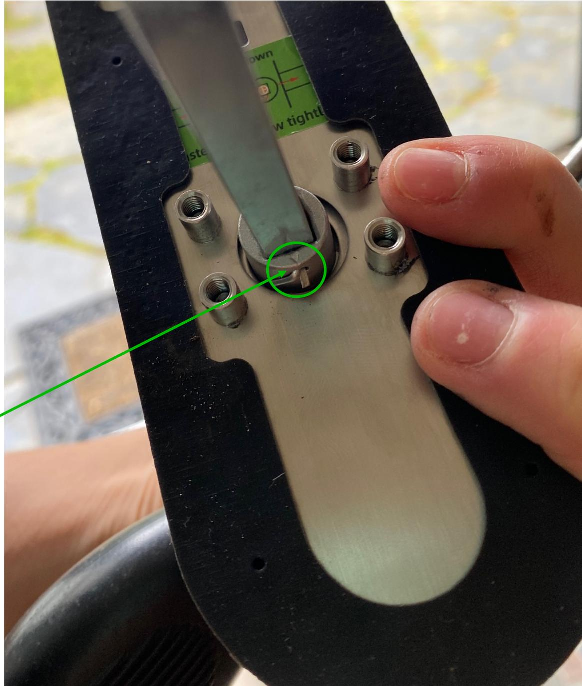
To secure that the motor of the lock is working properly, the arrow always needs to be pointing down when installing!
