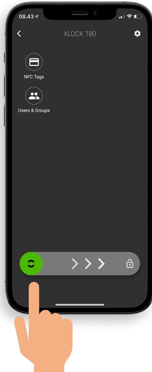
Unlocking with the smartphone and the app is very easy. A swipe to the right unlocks the lock. The reading distance is up to 15 meters. The lock can therefore also be hidden, e.g. installed behind a locker front, invisible. Toggle mode (open/close function) can also be used with the smartphone. This function is activated and deactivated in the lock settings.
