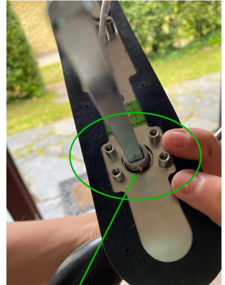
To secure the square shaft it is **very important** to bend the u-clip with the help of a screwdriver.
