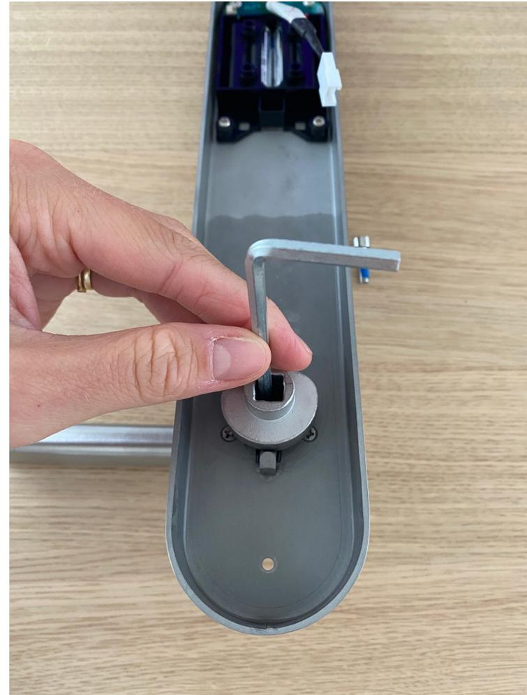
3. After adjusting the direction of the handle, insert it into the handle seat and re-lock the hexagon screw of the handle to complete the turning.
