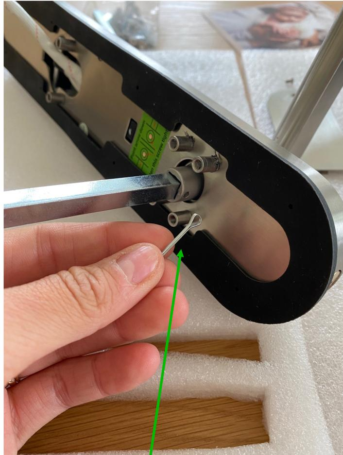
Make sure the rubber plate is installed on the front panel.
