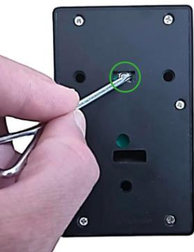
If you do not see the lock in the XL Lock Manager App search list after inserting the batteries, you can do a hard reset of the lock. To do so, press the reset button as shown on the picture for 3 seconds until a long sound arises. After the sound, the lock will be shown in the App, ready to be initialised.
