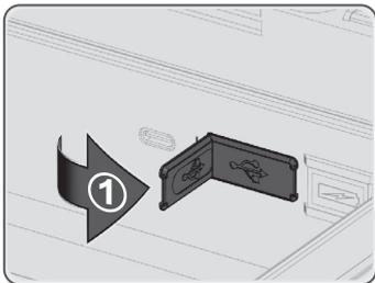
Devices connected to the USB port are supplied with power. Any device that uses more than 3 A of DC electrical current will trip a self-resetting function and disable the output.
