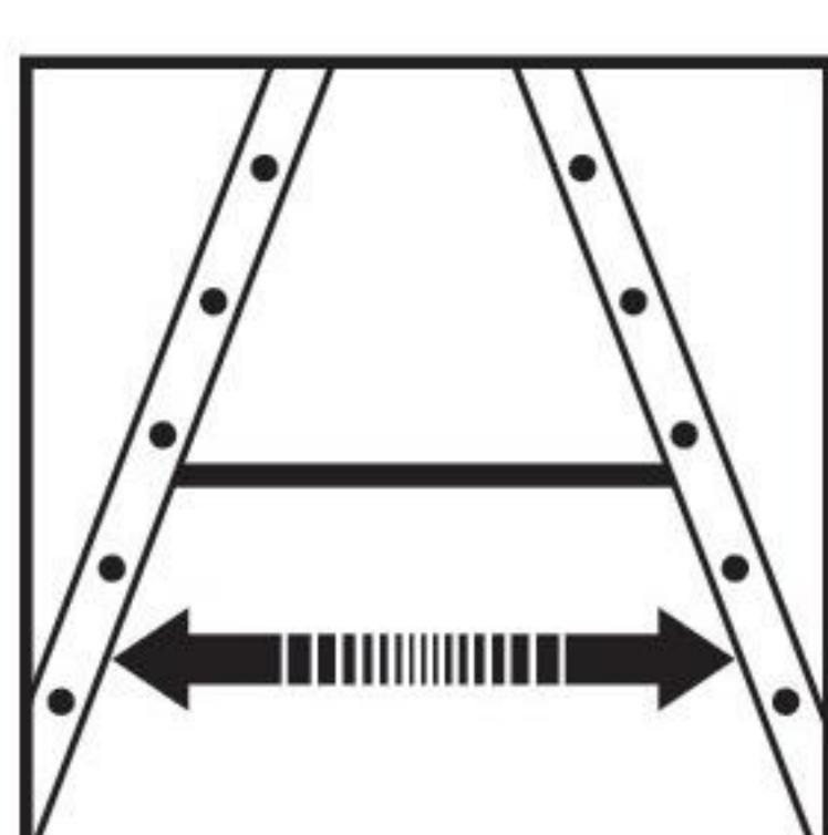
Ladder must be opened completely before use (bracing/bands should be fully opened, tightened/locked)
