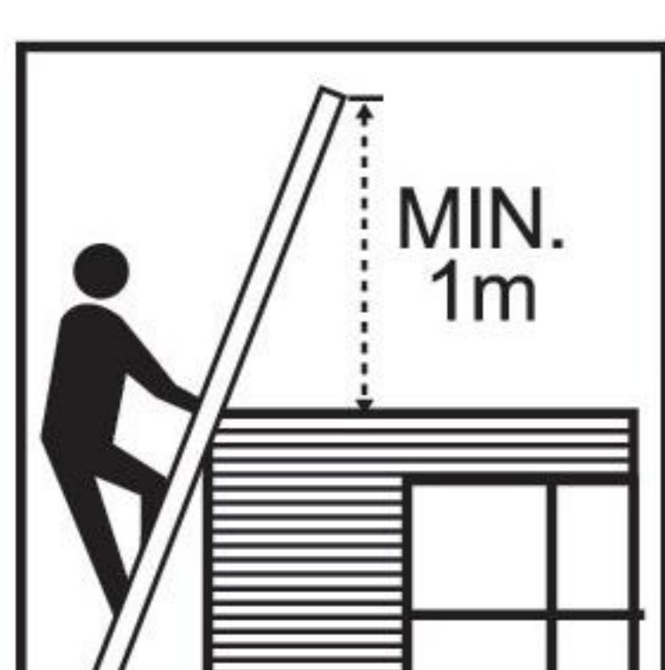
When used to access another level, ladder must extend min. 1 m over the landing point.
