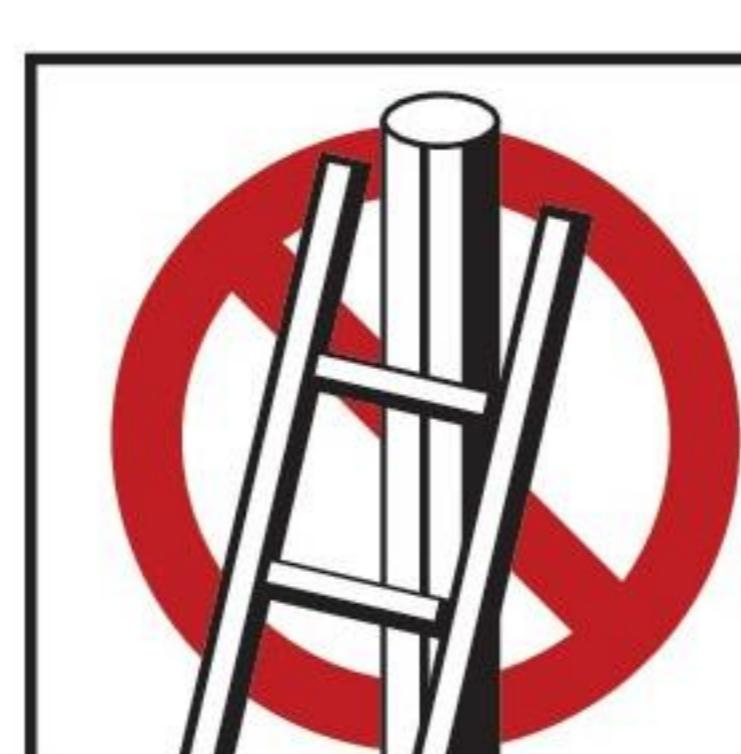
Ensure top of ladder is correctly positioned (ladder must always rest on both stiles - not the rungs)
