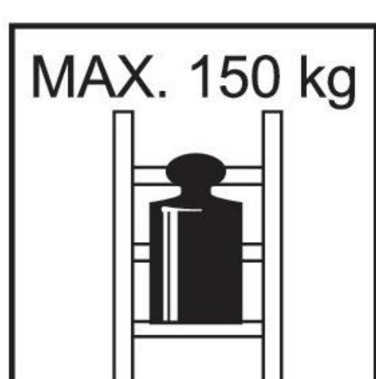
Max. load for the ladder is 150 kg.
