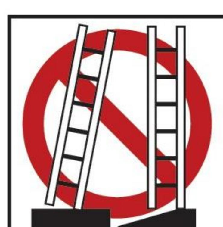
Erect on level base with ladder resting on both feet.
