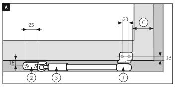
Assembly holes (in mm) apply for left, right, top and bottom. Note the hinge side.
