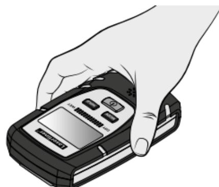
Always hold and press down the measuring device in the same way (see illustration).
