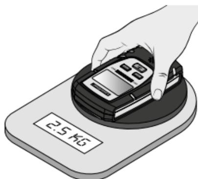
Place the device such that the sensor pads fully rest on the material to be measured and exert a pressure of about 2.5 kg onto the surface to be measured. **TIP:** Use scales to test the contact pressure.
