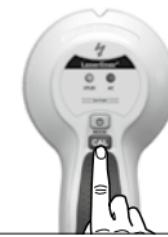
**!** The device and the wall must maintain contact during calibration in STUD-SCAN mode and throughout the entire measurement process. A hand should remain at the device the entire time as well.
