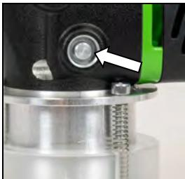
Press the spindle lock button to lock the work spindle.
