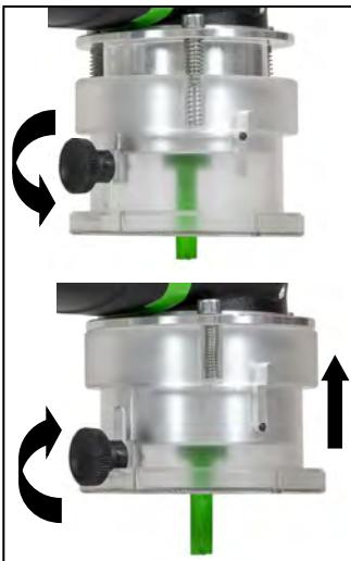
To adjust the milling depth, open the knurled screw on the protective cover. Push the spring-loaded ring of the protective cover as far back as it will go until the milling tool protrudes from the cover to the desired milling depth. Hold the ring in this position. Push the loosened cap, together with the knurled screw up to the stop (in the direction of the machine) and tighten the thumb screw.
