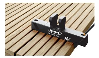
4. Place the screws in the pre-drilled holes which should have an angle of 50°. The process can be done with a placed Drill Tool 50X and without one. Start with the screw in the opposite direction (see the picture below).
