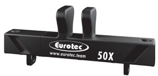
Through the help of fixation points the screws will be screwed in evenly in a 50° angle and are optimally placed. The spacer on the Drill Tool 50X will automatically create an equally joint gap of 6 mm between the different planks.
