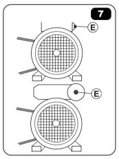
• NOTE: On the models equipped with an "OIL CONTROL" system, a power-off event may also be due to low oil level (see par. 4.5). Check oil level through the suitable oil window before resetting the relay.
