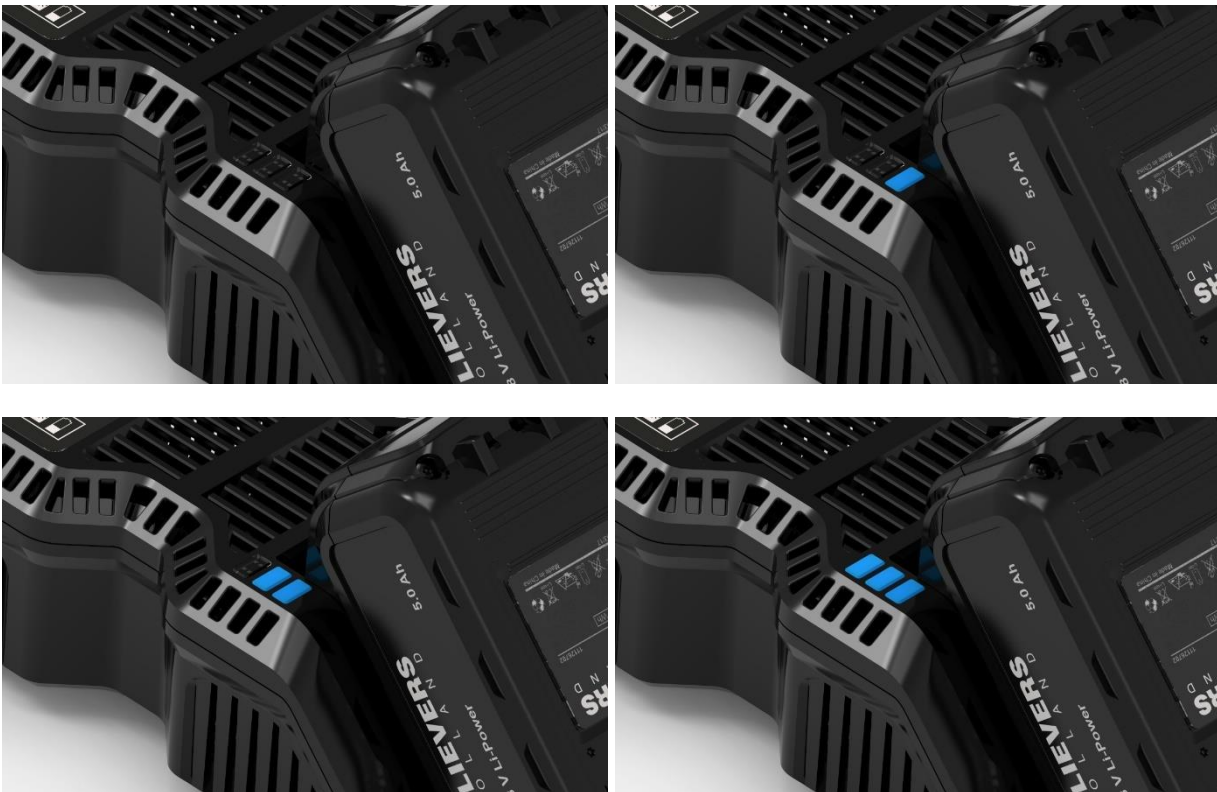
Figure 10: Charging a completely empty battery pack.
