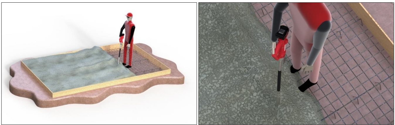
Figure 6: Compacting process during concrete.
